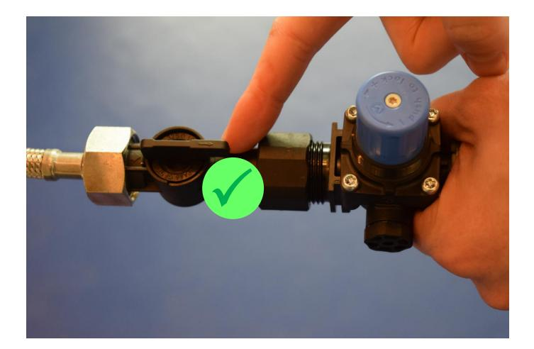
Close the locking handle of the filter head Now, the filtrate production will restart Check the system for leakages **BRITA**
